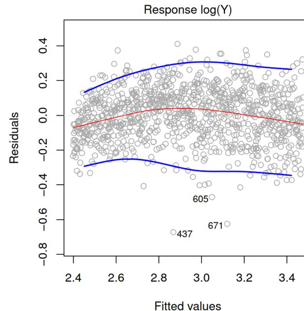
The right-hand panel displays the residual plot after transforming the response using log Y
