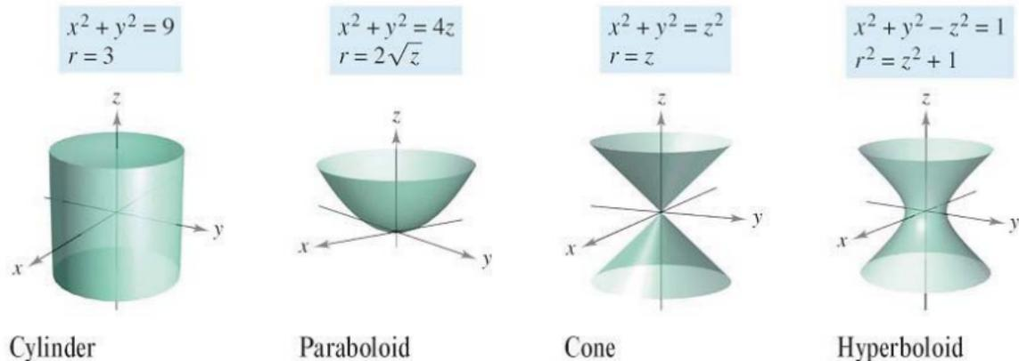
Figure 11: Different cylindrical equations.
