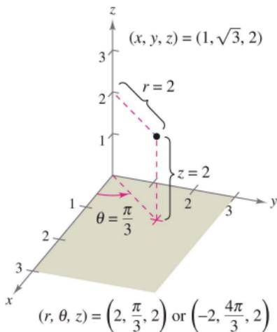
Figure 10: Converting from rectangular to cylindrical coordinates.
