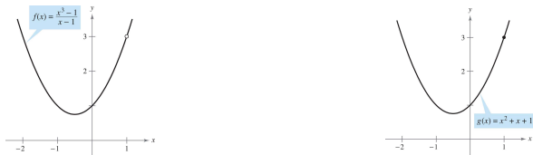
Figure 14: f(x) = \frac{x^3 - 1}{x - 1} , x \neq 1 and g(x) = x^2 + x + 1 agree at all but one point.
